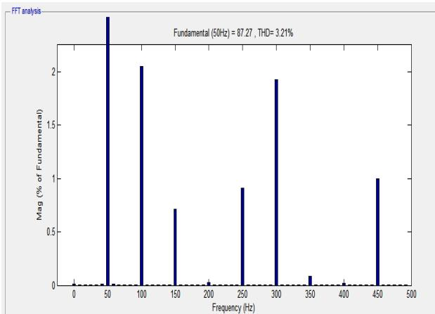
**Figure4.3:** Fast Fourier Transform(FFT)analysis for HCBMLI Fast Fourier Transform (FFT) analysis of HCBMLI is show in figure 4.3. Total harmonic istortion is 3.21% with a fundamental frequency of 50 Hz for its output voltage. The proposed topology is better when compared to the existing topologies.
