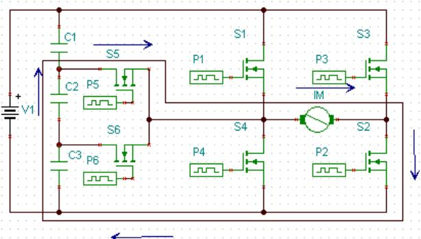
Figure 2.3 Mode II operation of MCHB Inverter
