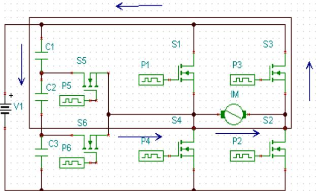
**Figure 2.6** Mode V operation of MCHB Inverter
