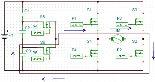
**Figure 2.4** Mode III operation of MCHB Inverter.
