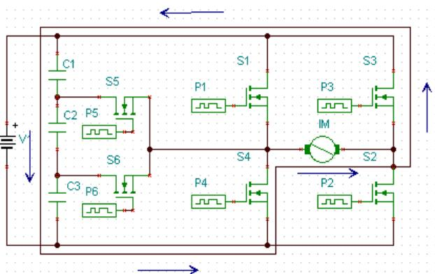
**Figure 2.7** Mode V operation of MCHB Inverter
