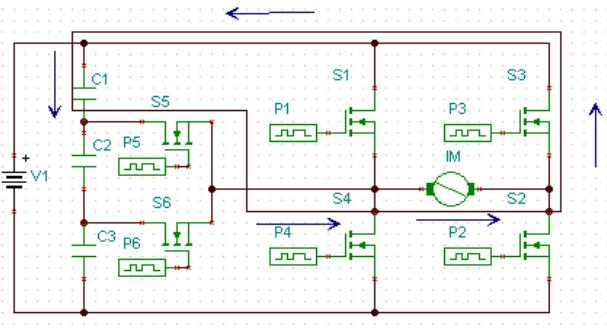
**Figure 2.5** Mode IV operation of MCHB Inverter
