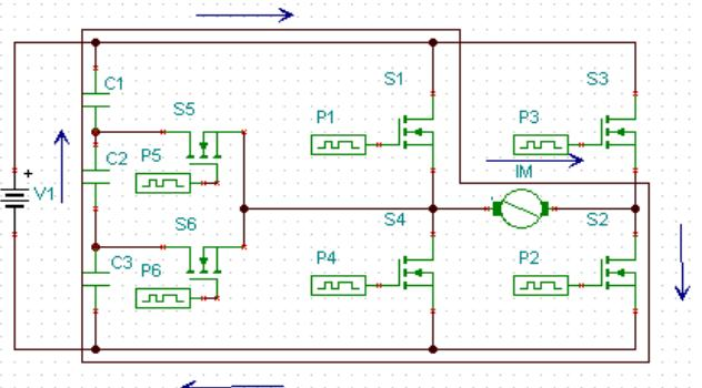
Figure 2.2 Mode 1 operation of MCHB inverter
